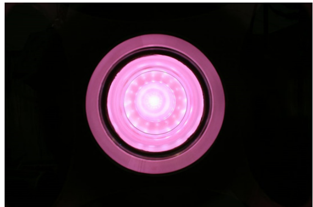
Fig.8 You can see the location of 20 plasma guns on the outer diameter of the Helion Energy setup and formed with theta-pinch FRC in the center.
