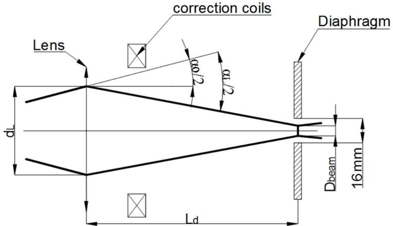
Fig.2.  $d_L$  is the diameter of the beam in the lens,  $D$  – measuring diaphragm with a hole diameter of 16 mm,  $D_{beam}$  is the measured beam diameter in the diaphragm,  $L_d$  is the distance from the lens to the diaphragm, which is 940 mm.
