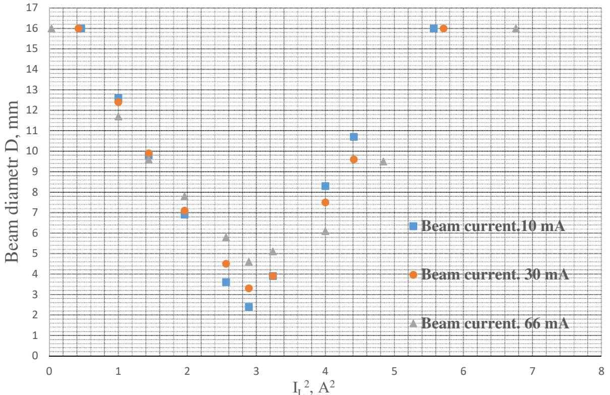
Fig.1. Dependence of the beam size in the diaphragm on the focusing lens current at an energy of 1.5 MeV.
