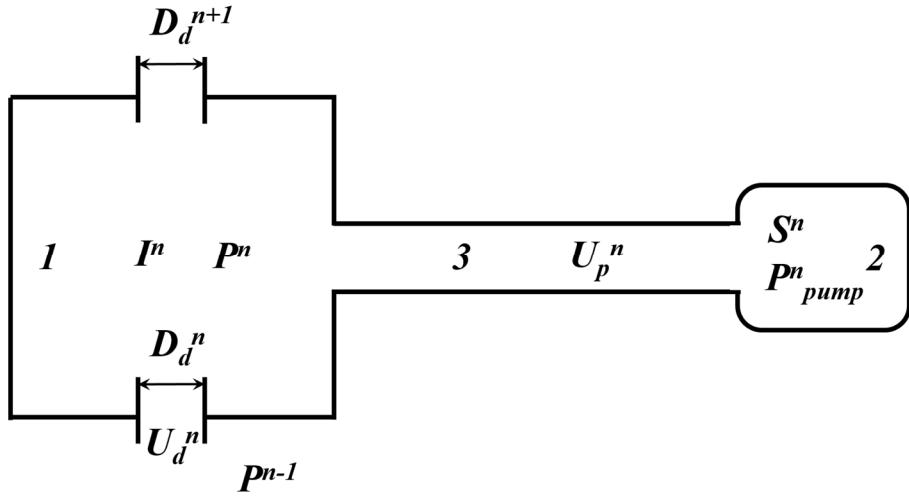
Fig.3. Diagram for the vacuum calculation of the differential pumping stages: 1 – chamber; 2 – pump; 3 – tube.
