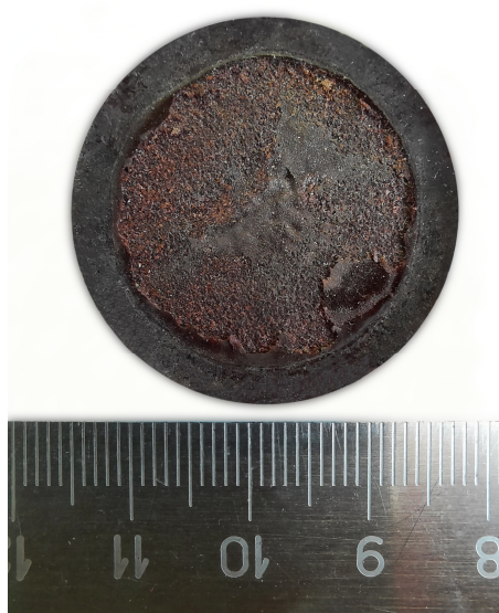
Fig.7. Irradiated rubber sample. Beam energy 350 J.
