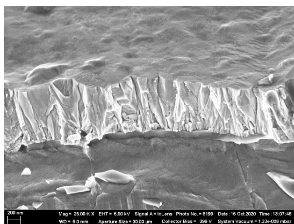
Fig.3. SEM image of the transverse cleavage of the coating deposited under ion current density of 1 \text{ mA/cm}^2 .
