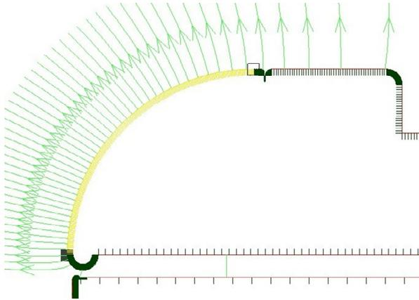
Fig.3. Electric field strength at the high voltage electrode.
