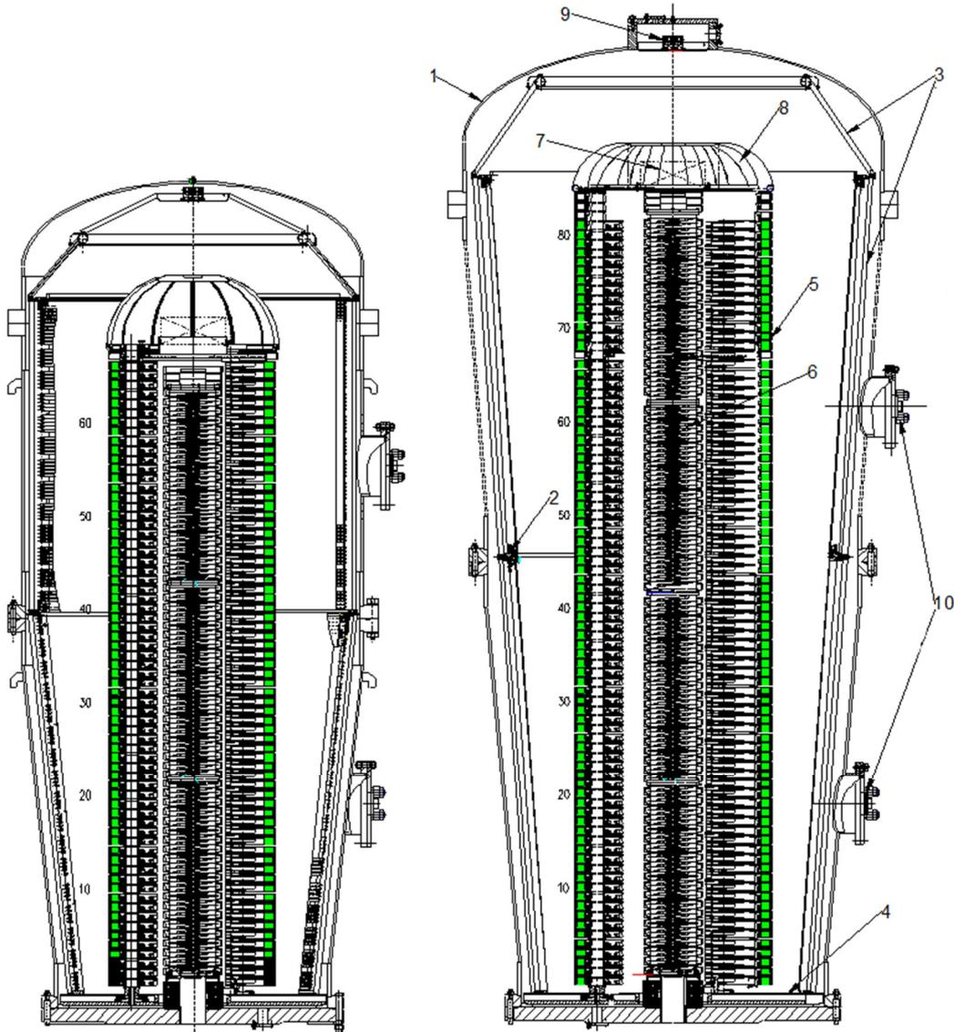
Fig.1. ELV-8 (left) and ELV-15 high voltage rectifiers. 1 – vessel; 2 – primary windings; 3,4 – magnetic circuits; 5 – rectifier sections; 6 – accelerating tube; 7 – injector control unit; 8 – high voltage electrode; 9 – rotary voltmeter with capacitance probe; 10 – primary winding terminals.
