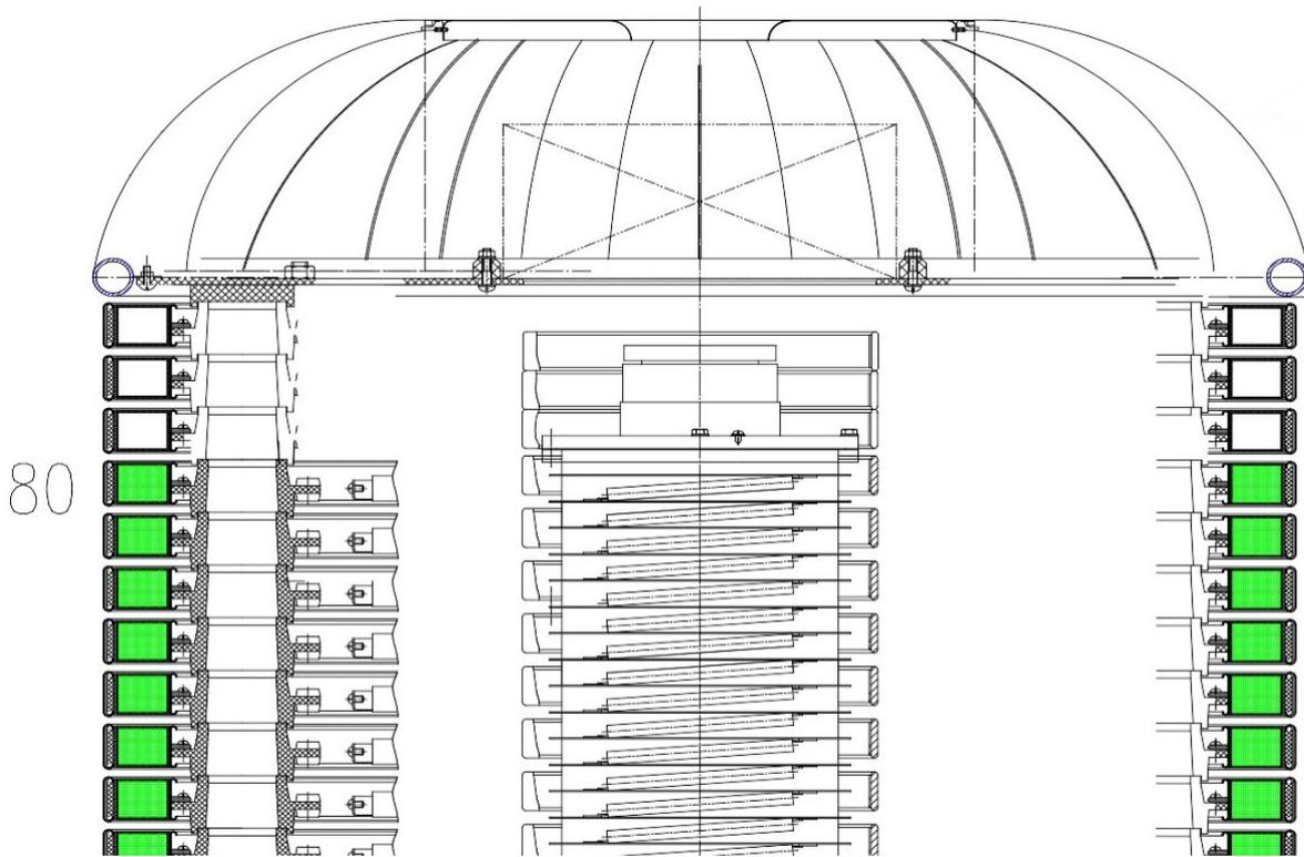
Fig.2. High voltage rectifier column with three “empty” sections on top.
