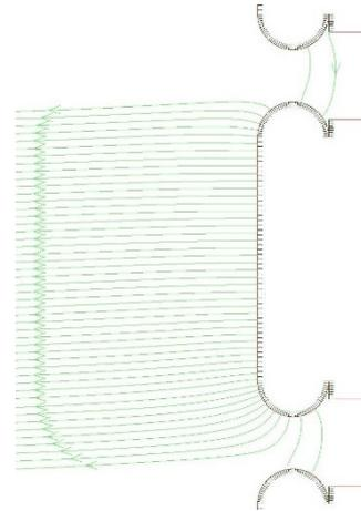
Fig.4. Electric field strength at the screen of rectifying section.
