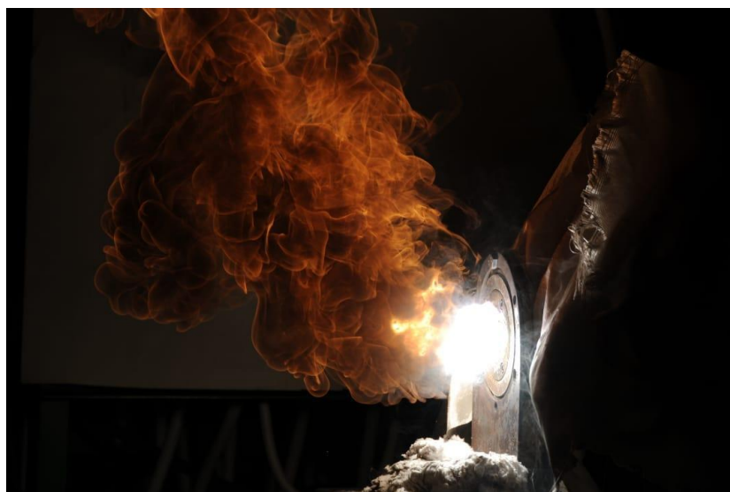
Fig.1. High-voltage AC plasma torch.
