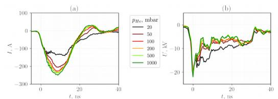
Fig.2 Oscillograms of current (a) and voltage (b) at different nitrogen pressures
