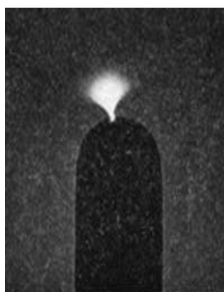
Fig.3. Typical images of corona glow on the cathodes of different diameters. L. B. Loeb, Electrical Coronas , Univ. of California Press, Berkley, USA (1965)
