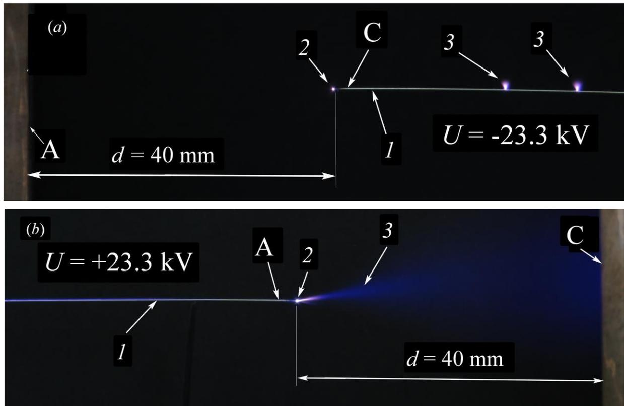
Fig.1. Photographs of the glow of a corona discharge, demonstrating different modes in a gap 40 mm long with negative (a) and positive polarity of the tip (b). 1 - needle, 2 - area of bright glow at the tip of the needle, 3 - plasma jets.
