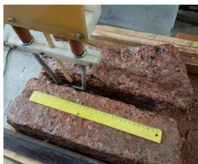
Fig.1. Photograph of a cut slit in granite.
