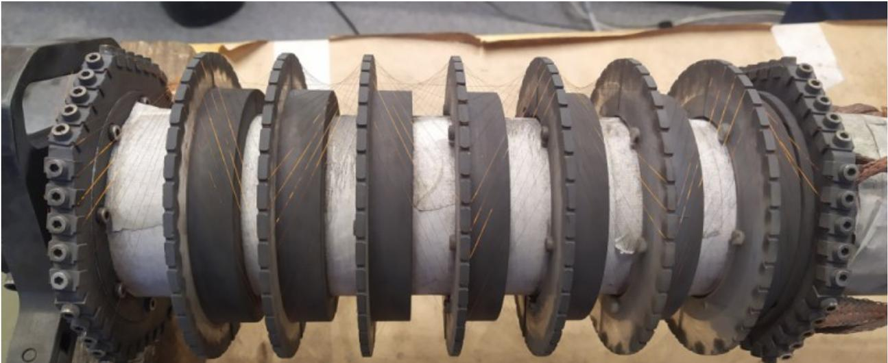
Fig.1. Exploding wire array with zigzag wires installation.
