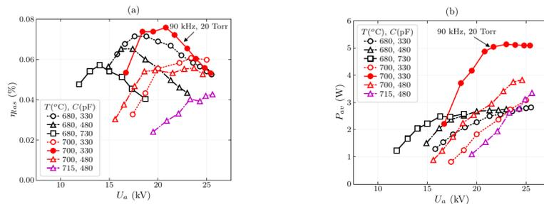
Fig. 1. Dependences of the laser efficiency  $\eta$  (a) and average output power  $P_{av}$  (b) on the voltage amplitude  $U_a$  at the operating capacitance for different values of the operating capacitance  $C$  and GDT wall temperature  $T$ . Helium buffer gas pressure  $p$  equals 10 Torr and PRF  $f = 50$  kHz, except for the curve with maximum values.
