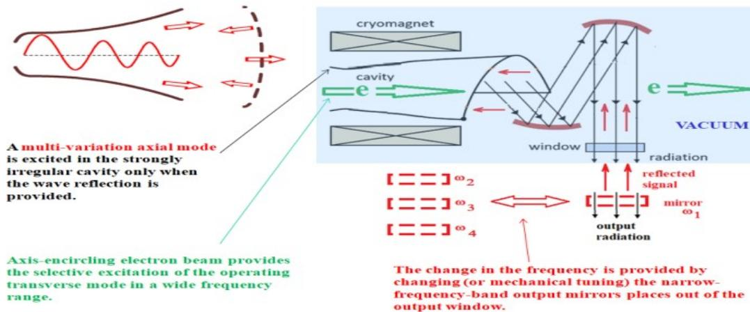
Fig.1. Schematic of the gyrotron with reflections of the excited wave from the external frequency-tunable mirror.
