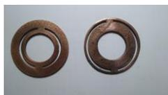
Figure 2- Split rings printed and copper plated
