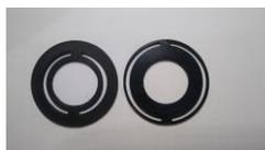
Figure 1- Split Rings printed with conductive material
