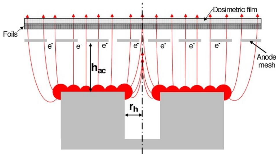
Fig.1. Electrostatic cumulation.
