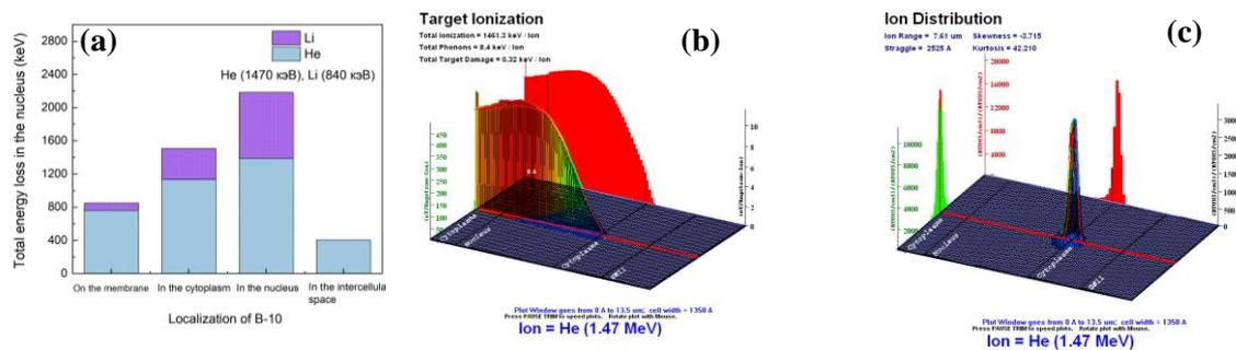
Fig. 1. Simulated radiation damage to tumor cells. (a) – the total energy loss on the ionization of the nucleus (violet and blue colors correspond to energy loss by Li ions and  $\alpha$ -particles, respectively), (b, c) – Interaction of  $\alpha$ -particles (1470 keV) with the cell during BNCT when BNQDs were localized in the cell cytoplasm: (b) – ionization of the target itself during the propagation of  $\alpha$ -particles, (c) – final distribution of  $\alpha$ -particles in the target.
