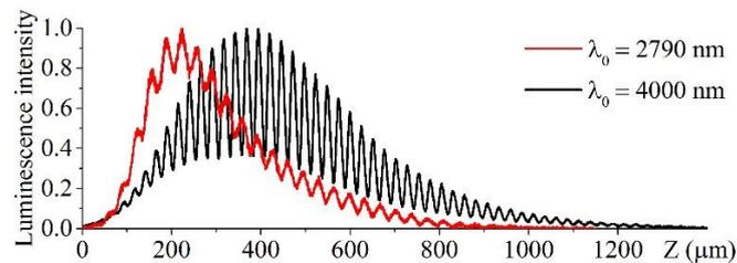
Fig.1. Experimentally measured luminescence profiles on the axis of tracks of color centers induced in LiF by a light bullet at wavelengths (red curve) 2790 nm, (black curve) 4000 nm.
