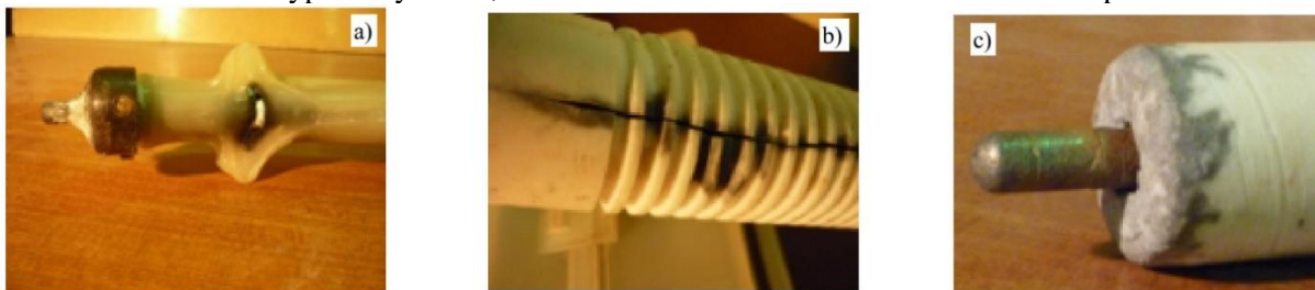
Fig 1. Types of destruction of the high-voltage electrode insulator
