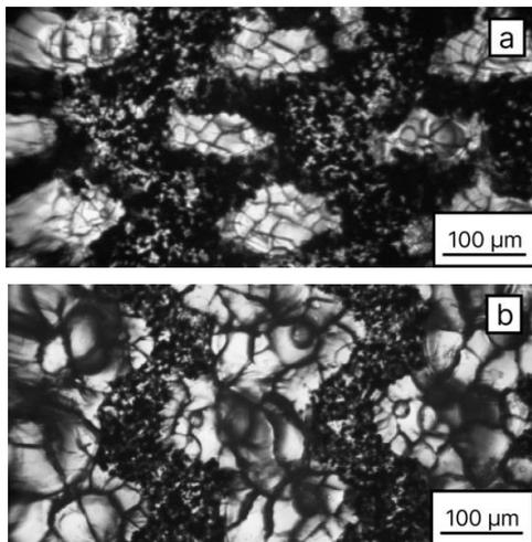
Fig.1. Micrographs of the surface of samples laser-treated at  $E_{pulse} = 14$  mJ (a) and 38 mJ (b).
