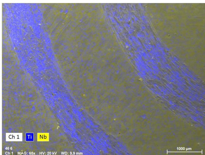
Fig.1. Surface EDS map of the Al<sub>2</sub>O<sub>3</sub> ball trace left on Ti-Nb wear tests on sample synthesized with 100 nm of deposited Nb and LEHCEB alloyed at 25 kV with 10 pulses.
