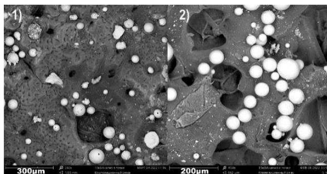
Fig.2. Spherical particles of iron oxide photographed through a Phenom ProX electron microscope obtained with EEW(1) and LA(2).
