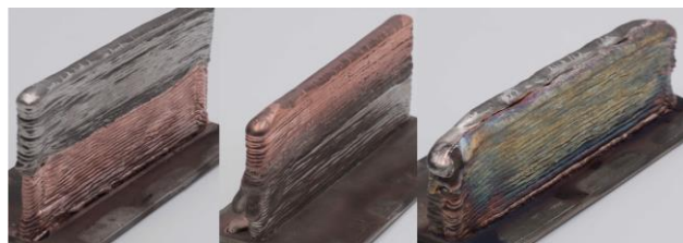
Fig.1. Ni-Cu bimetallic products obtained by EBAM.
