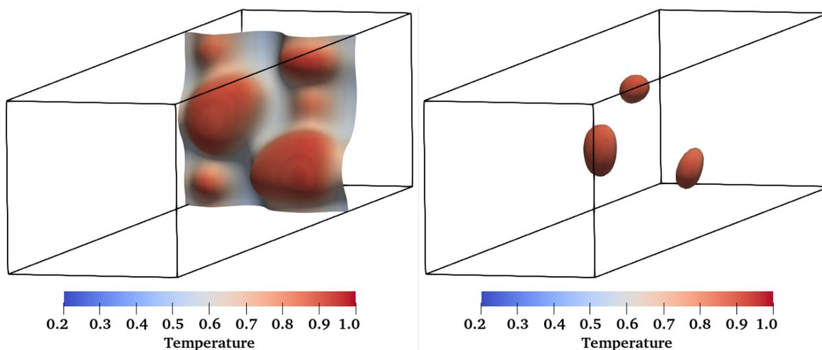
Fig.1. Isosurfaces of the concentration  $C=0.1$  colored according to the gas temperature and illustrating the surface of the reaction front in straight channels: continuous cellular flame front (on the left) and sporadic combustion wave (on the right).
