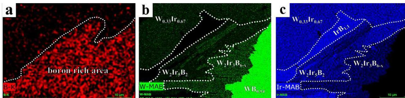
Fig.1. Mapping by cross-section elements of a powder mixture of iridium and tungsten boride (3:1) heated at 1600 °C:
