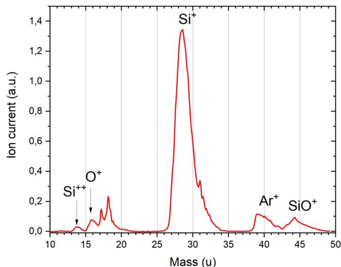
Fig.1. Mass spectrum of ion flux from HiPIMS discharge on Si target in O<sub>2</sub>/Ar.
