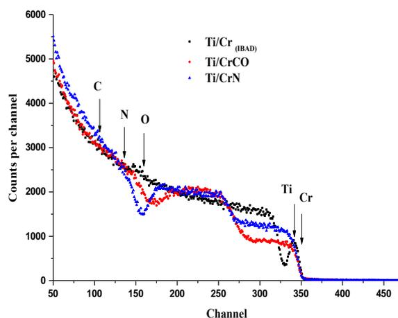
Fig. 1. RBS spectra of  $^4\text{He}$  ions scattered by atomic nuclei of elements that make up titanium surfaces with layers formed by: chromium IBAD ( $\text{Ti}/\text{Cr}_{(\text{IBAD})}$ ); ion-plasma deposition of chromium oxycarbide ( $\text{Ti}/\text{CrCO}$ ) and chromium nitride ( $\text{Ti}/\text{CrN}$ ).
