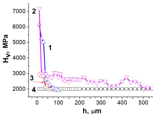
Fig. 1. Microhardness profiles of AISI 1020 steel samples subjected to nitriding at temperatures of 600 $^{\circ}\text{C}$  (curve 1), 520 $^{\circ}\text{C}$  (curve 2), and 450 $^{\circ}\text{C}$  (curve 3); curve 4 - AISI 1020 steel in the initial state
