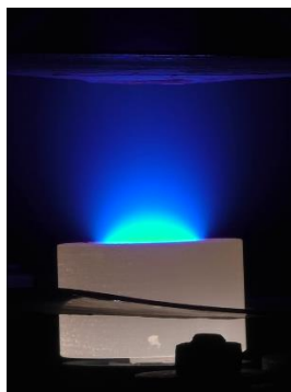
Fig.1. Photo of the diffuse vacuum arc discharge on mixture cathode of CeO 2 and Cr powders.
