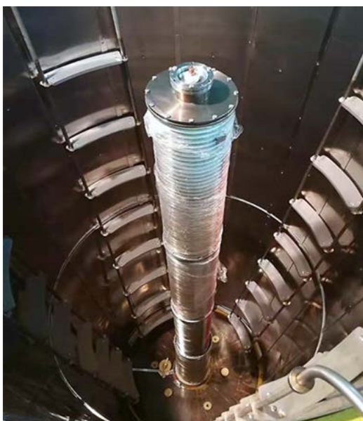
Fig.1. Accelerating tube inside of primary windings of ELV-15 accelerator.
